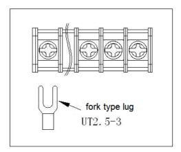
Figure 5-2 Connection Diagram of Main Terminal
