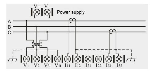
Figure 5-5 Wiring Diagram of 3-phase-3-wire
