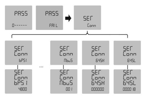
Figure 4-2 Parameter Setting with Keys
