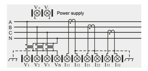
Figure 5-4 Wiring Diagram of 3-phase-4-wire (With PT)
