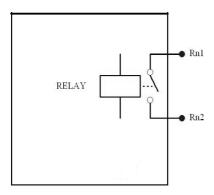
Figure 3-3 Circuit Diagram of Relay Output Interface
