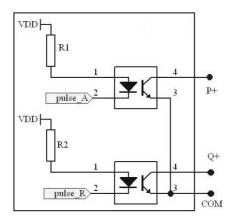
Figure 3-1 Circuit Diagram of Power Pulse Output Interface
