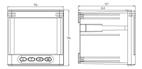
Figure 5-1 Total Dimension of Instrument
